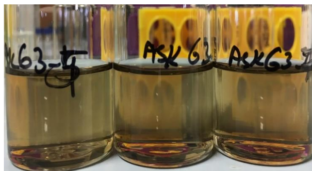
Figure 1.33. Photograph of the reaction mixture before destabilization with water, composed of Core-shell IONCs and PScMA that are dissolved in THF.
