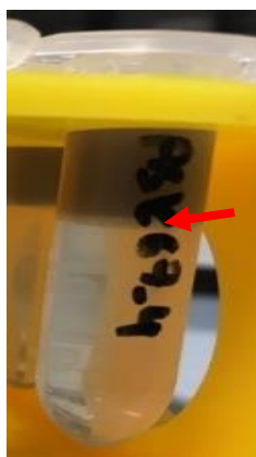
Figure 1.12. A photograph of sample under washing. The upper dark water phase composed of nanoclusters, which is indicative for their water transfer. The unreactive polymer can be identified at the interface as dense whitish substance (red arrow). While the lower clear solution is \text{CHCl}_3 phase.
