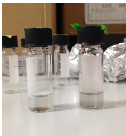
Figure 4.24 Suspensions of GO-AB1 and GO-AB2 in 50 \mu\text{g}/\text{mL} in \text{H}_2\text{O} after 10 min of sonication.
