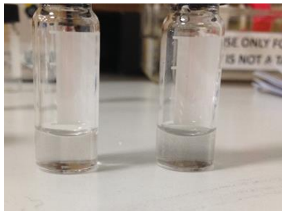
Figure 4.23 Suspensions of GO-AB1 and GO-AB2 in 50 \mu\text{g}/\text{mL} in \text{H}_2\text{O} after shaking.
