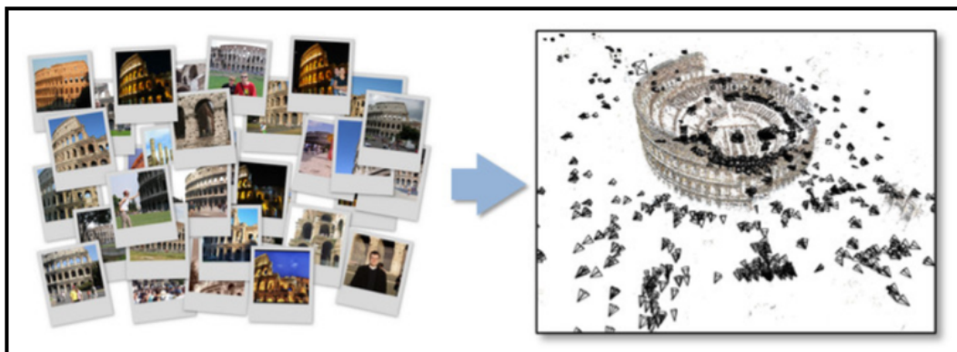
Figure 1.7: An example of Structure from Motion methods. Bundler [1] reconstructing the scene from unordered photos obtained from internet.
