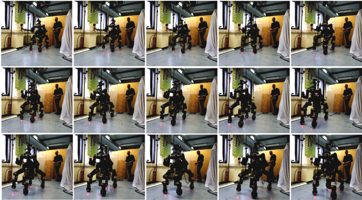
Figure 6.6 Snapshots taken from an experiment on the actual CENTAURO robot. For the sake of clarity, the final backward phase is not included.
