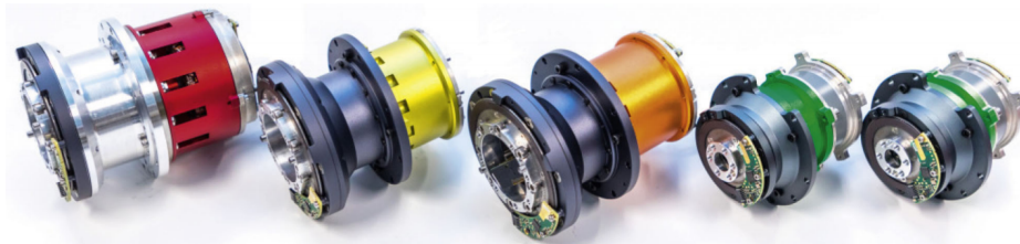
Figure 1.5 Torque controlled integrated actuators used inside HHCM robots. Different sizes, when combined with different transmission ratios, allow to select a trade-off between weight, speed and torque.
