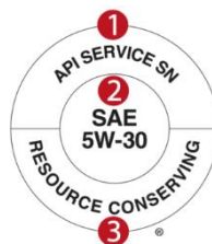
Figure 3.1: API "Donut": 1) This part displays the motor oil's API performance standard; 2) The centre of the "Donut" shows the motor oil's SAE viscosity grade; 3) The bottom tells whether the motor oil has resource-conserving properties when compared with a reference oil in an engine test.
