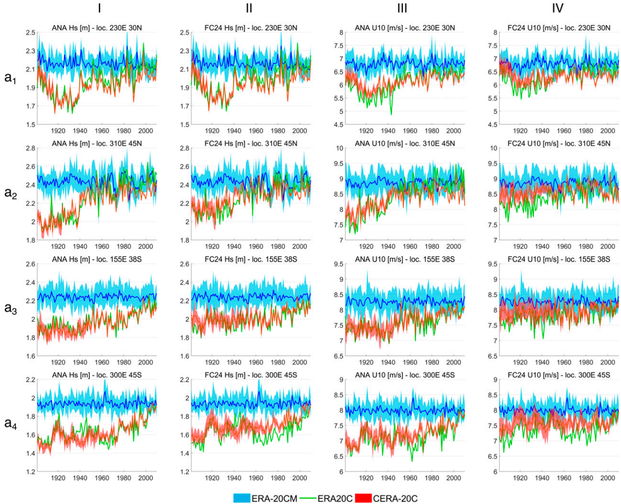
FIG. 5. Yearly averages of monthly mean values at four different locations indicated in Fig. 4b. For ERA-20CM and CERA-20C, the envelope of the ensemble values are plotted together with the mean. Columns represent (left to right) ANA H_s , FC24 H_s , ANA U_{10} , and FC24 U_{10} , respectively.
