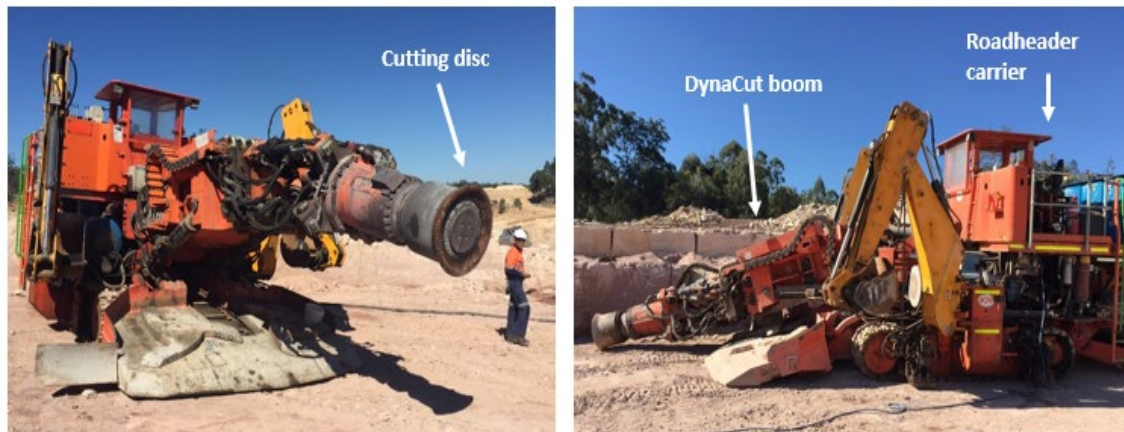
Figure 3: Main test equipment- modified roadheader with DynaCut cutting systems
