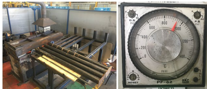
Figure 2: DSI Martin Furnace with test pieces (left) and max. furnace temperature (right)
