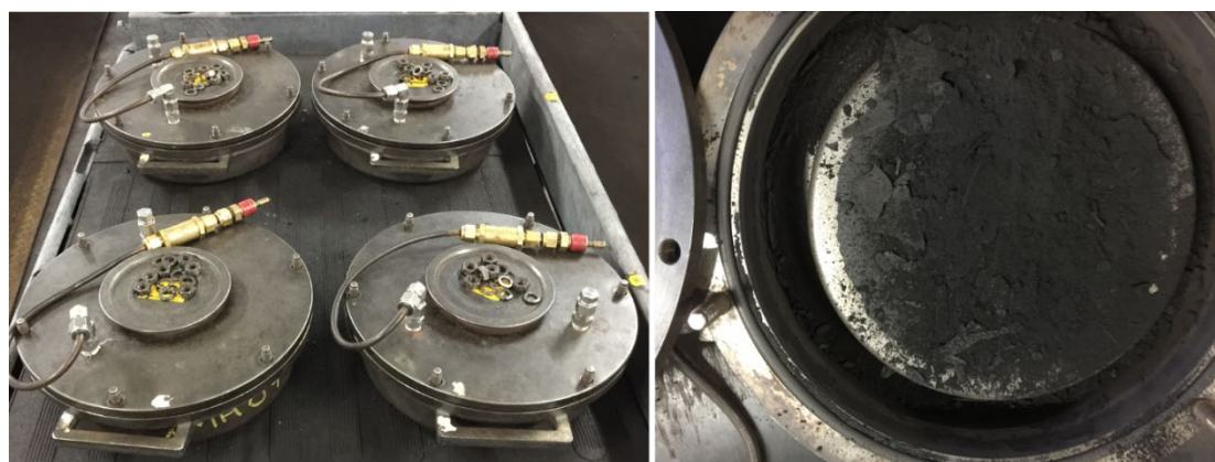
Figure 5: Ring mill crushers for Q3 residual gas content measurement and pulverised coal
