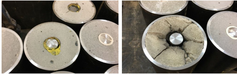
Figure 10: 150 mm-long samples prepared for push-testing (top), uncatylsed resin (bottom left), and heat-affected sample (bottom right)
