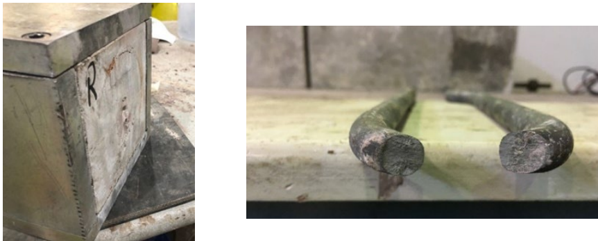
Figure 7: Test 3- Sheared surface of 16 mm rock bolt in a confined concrete The effect of friction
