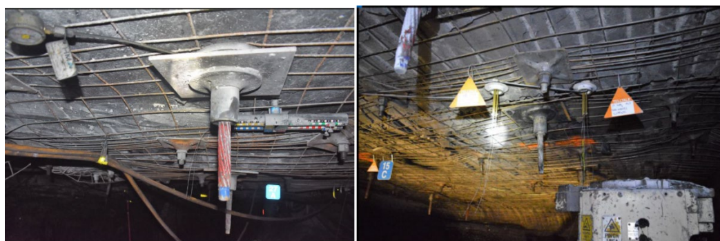
Figure 7: Load cell and extensometer monitoring configuration during implementation
