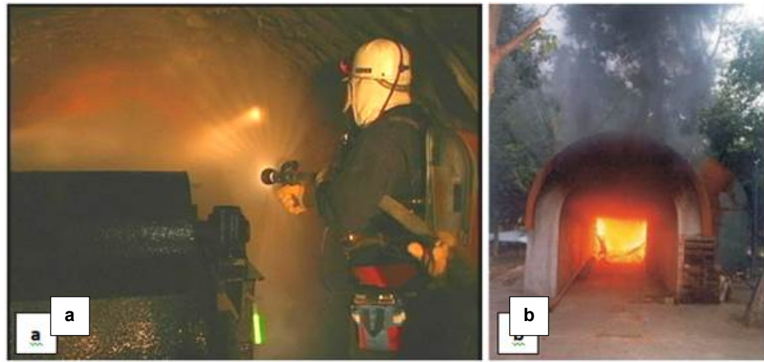
Figure 1: (a) rescue team fighting a conveyor belt fire (Conti 2001), and (b) Dhanbad fire test gallery (Singh and Ray 2005).
