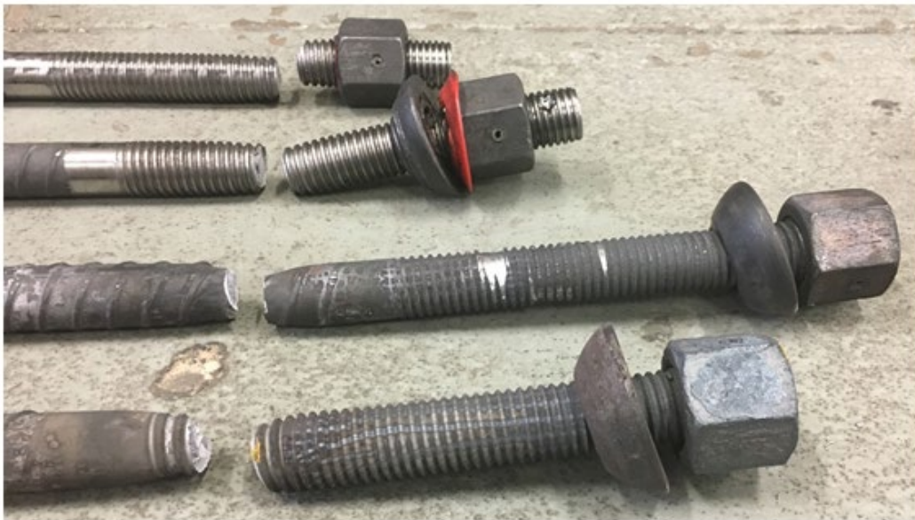
Figure 13: Bolts failed during tensile tests – non-heated at top and heated at bottom
