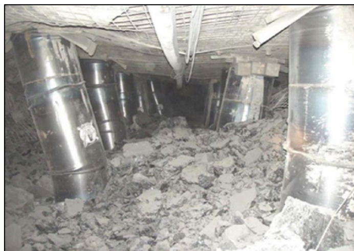
Figure 32. Elk Creek longwall tailgate coalburst (Mark 2016)
