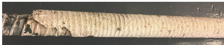
Figure 6: Example of the drill hole profile produced using a consistent drill feed rate
