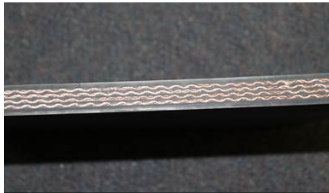
Figure 2: Sample of used conveyor belt that generated the CBRF, showing Polyester Nylon (PN) webbing embedded in rubber layers
