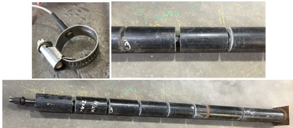
Figure 3: Thermocouples were fitted to a 1.8 m-long bolt installed in a grout-filled steel cylinder. Note the resin was removed to allow fitment of the thermocouple to the bolt steel.
