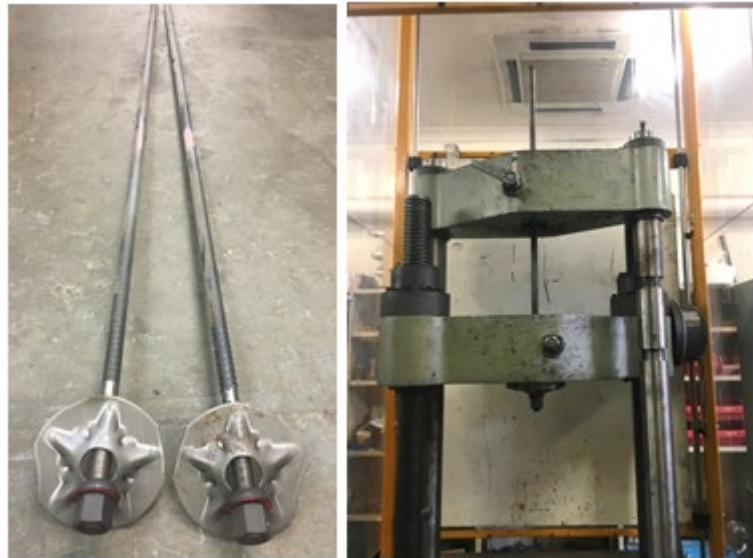
Figure 5: Tensile test arrangement of complete lower-anchor assembly comprising bolt, nut, dome and bearing-plate
