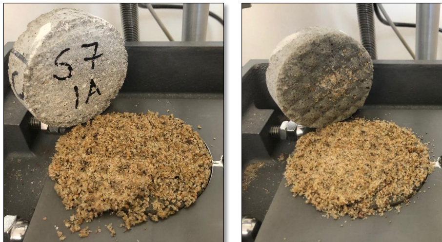
Figure 10: Sample A with infill height equal to asperity height
