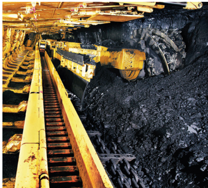
Figure 3: Longwall face equipment
