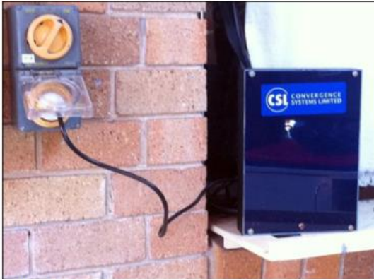
At each participating school, Tonge installs several CSL RTLS RFID anchor readers, each plugged into a power source.
