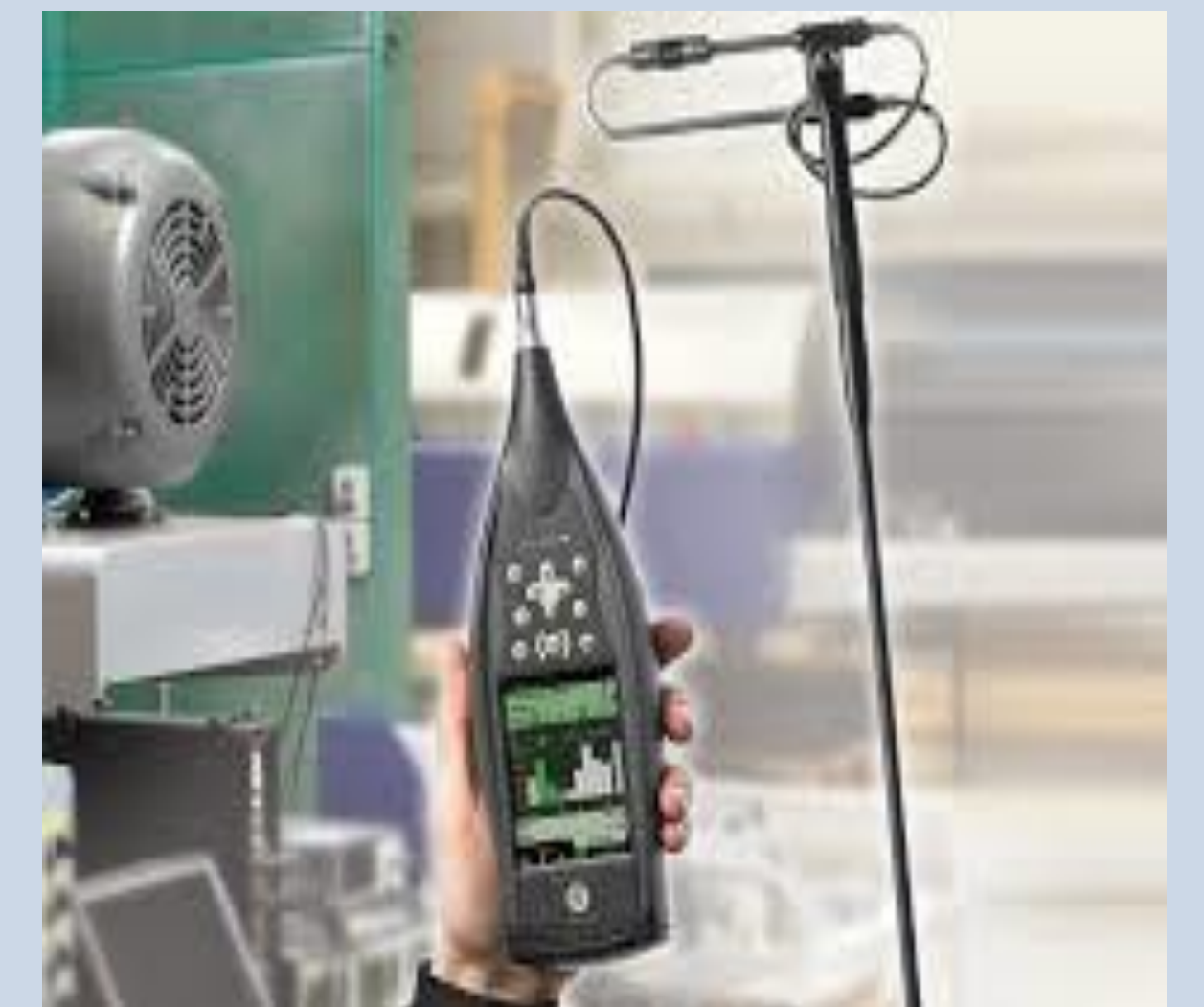
Fig 6. Demonstration of Sound Intensity used for measuring fan's sound power levels, image courtesy of Bruel & Kjaer
