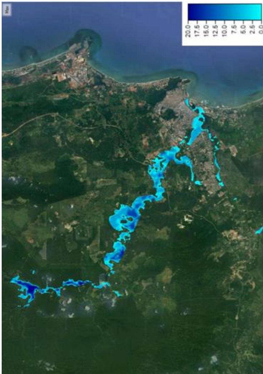
Figure 9. The inundation mapping due to Chereh Dam failure during heavy rainfall with 100 years ARI
