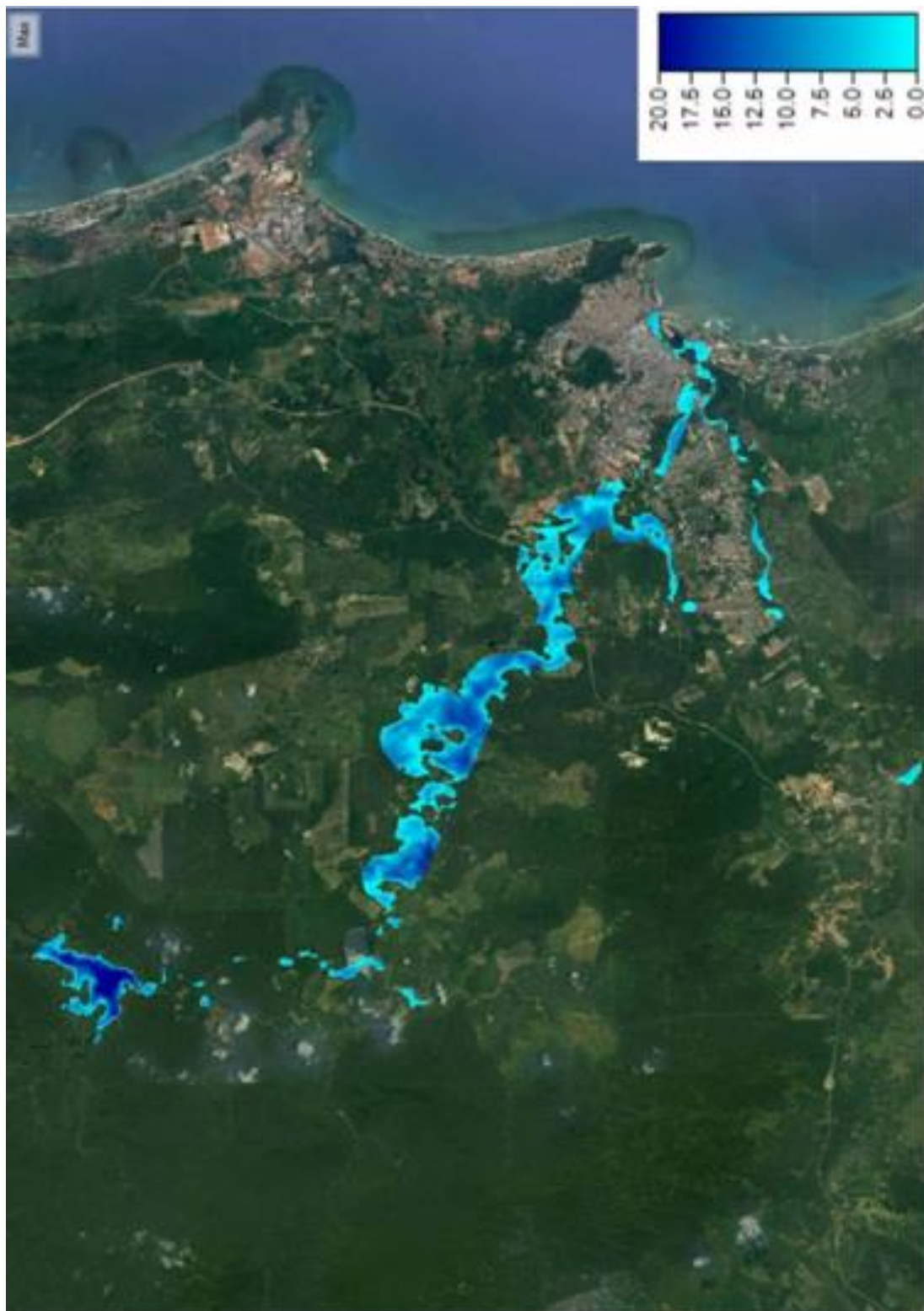
Figure 8. The inundation mapping due to Chereh Dam failure during heavy rainfall with 50 years ARI
