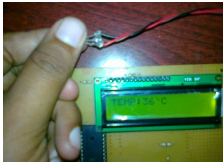
Figure 10. Hardware for body temperature measuring.
