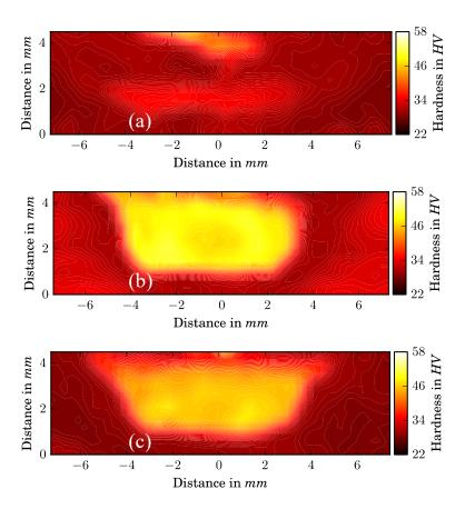
**Figure 7.** Hardness mappings recorded with a Berkovich indenter,  $500 \, mN$  indentation force and  $300 \, \mu m$  spacing between the indents. Sample 1 (a), sample 2 (b) and sample 3 (c)
