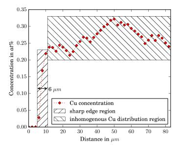
**Figure 5.** EDX line scan of Cu concentration of sample 2 at the position marked in Figure 2. The strongly fluctuation concentration profile inside the mechanically alloyed region as well as the clearly defined sharp edge is marked.
