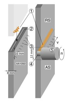
**Figure 1**. Schematic diagram of the sample production by a combination of Friction Stir Welding and Friction Stir Processing of the joint of two aluminium sheets with copper powder (1) in between. A groove (2) in the lower sheet is filled with commercially pure copper and the temperature during the process is measured by thermocouples (3). A rotating steel probe (4) with a shoulder (5) distributes the additional copper within the Aluminium matrix.
