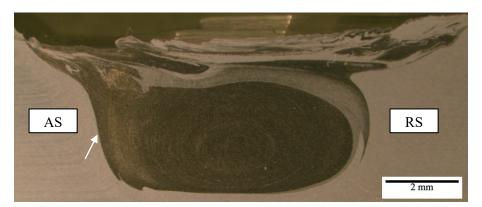
**Figure 2.** Macrograph of cross section of sample 2 taken with a light microscope after polishing and etching with Kroll's reagent. Advancing and retreating side of the second pass as well as the position of EDX analysis are marked.
