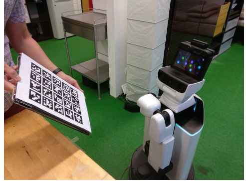
Figure 5.3: Demonstrating a trajectory to the HSR using a motion-capture imitation learning approach. Courtesy of Mitrevski et. al. ([76])
