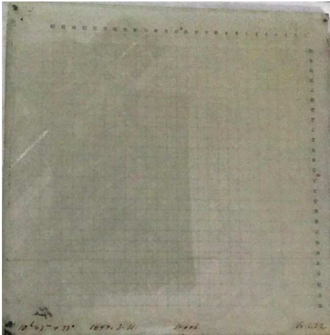
Fig. 1: Glass photographic plate from the Carte du Ciel survey, Potsdam Observatory, Plate 5, taken January 11, 1894. The plate is approximately 16 cm x 16 cm; each plate covered two square degrees of the sky, courtesy of the Leibniz-Institut für Astrophysik, Potsdam.
