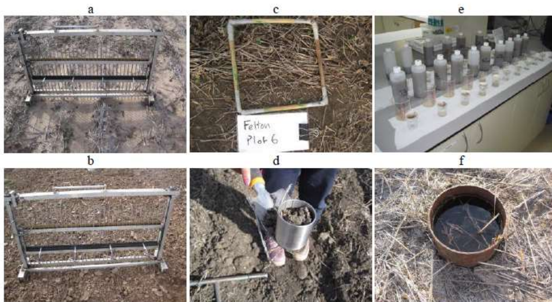
Figure 7: Instrumentation used to characterise rainfall simulation plots and treatments included profile microrelief measurements before (a) and after (b) tillage, biomass (c) and soil (d) collection, filtration of runoff samples (e) and single-ring infiltrometers (f).
