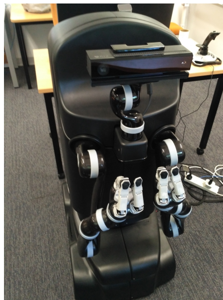
Figure 1.1: MOVO, a mobile manipulator by Kinova Robotics
