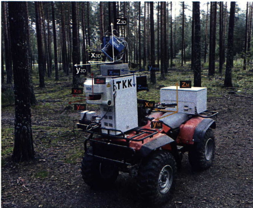
Figure 5: The all terrain vehicle with its relative coordinate systems is in the picture. Vehicle’s main coordinates are drawn with yellow, IMU coordinates with blue, 3D scanner coordinates with white, and 2D scanner coordinates with red color. The y-axis is pointing to the heading direction in all other relative coordinates except IMU coordinates.
