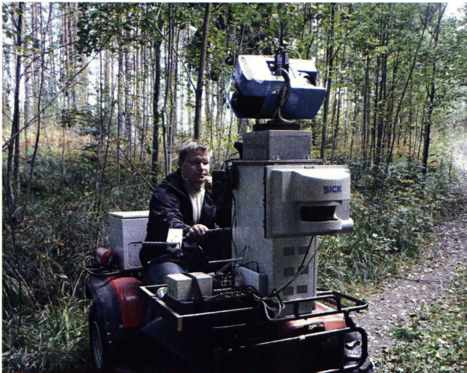
Figure 3: Image of the later version of the measurement vehicle at front. The horizontal 2D laser scanner was mounted to front of the system pointing forwards. The rotating 3D laser scanner is mounted on top of the vehicle. Researcher Mikko Miettinen is driving the vehicle in the picture.
