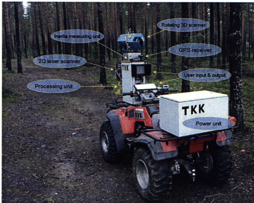
Figure 2: Honda all terrain vehicle and parts of the latest version of the measurement system. The difference between the initial and the latest versions is that the initial version had two 2D laser scanners pointing sideways in contrast to the latest version which has one 2D and one 3D scanner.
