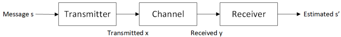
Figure 4.1: A simple wireless communication system consisting of a transmitter and a receiver through a channel.
