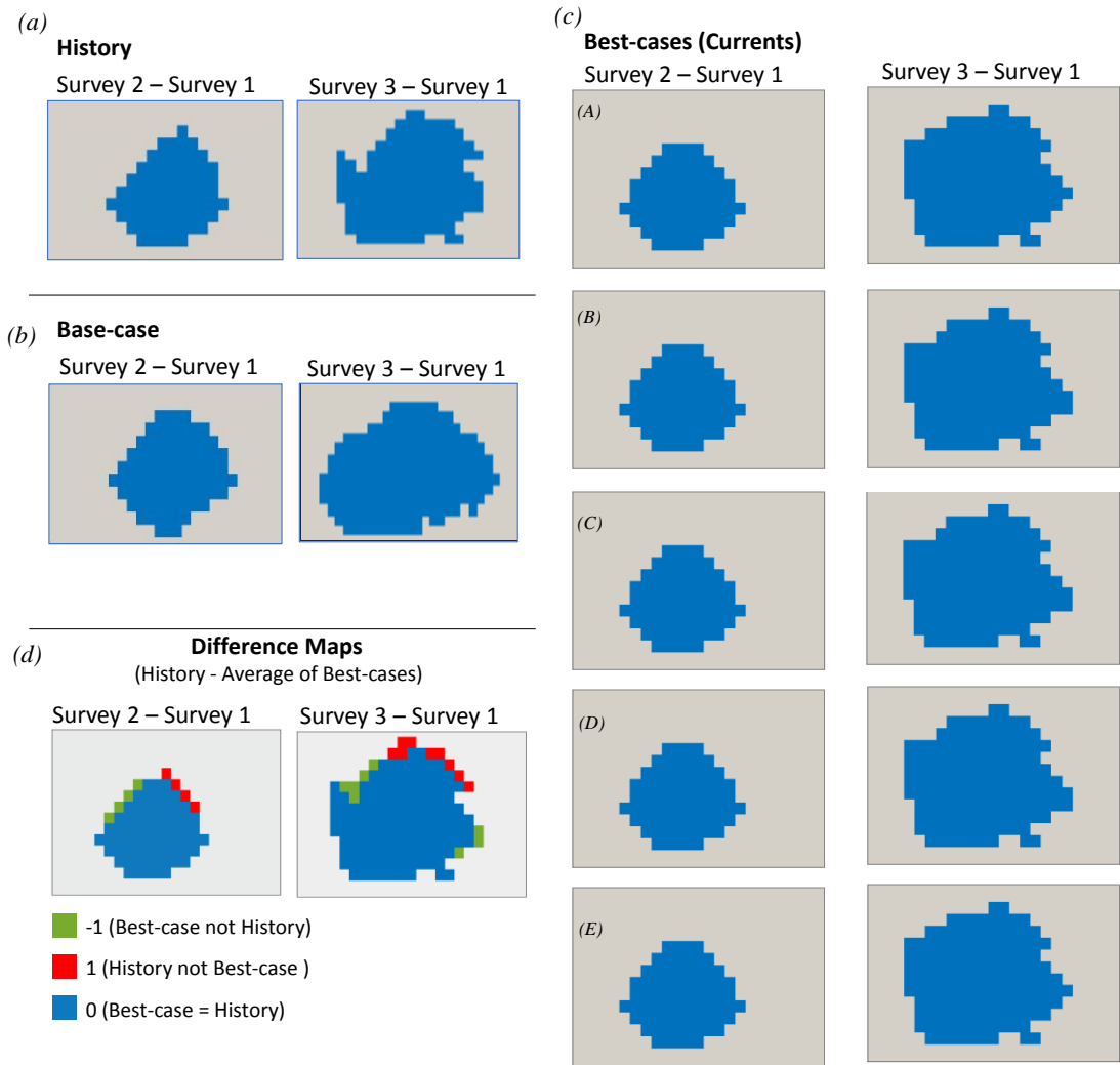
Figure 5.19: Binary maps comparing the maps from the observed (history) and base-case maps to maps from the best-case model as a result of history matching using Currents Measurement Metric method.
