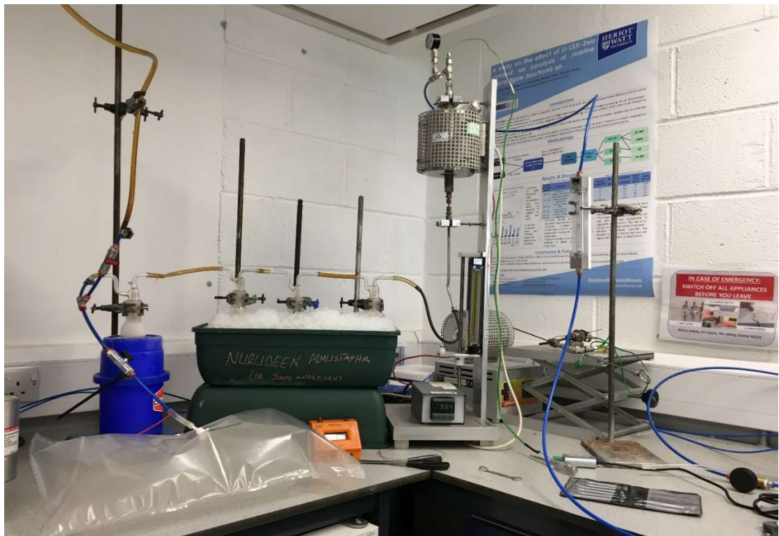
Figure 3-13 (a) Schematic diagram. (b) Real set-up of the vertical pyrolysis set-up
