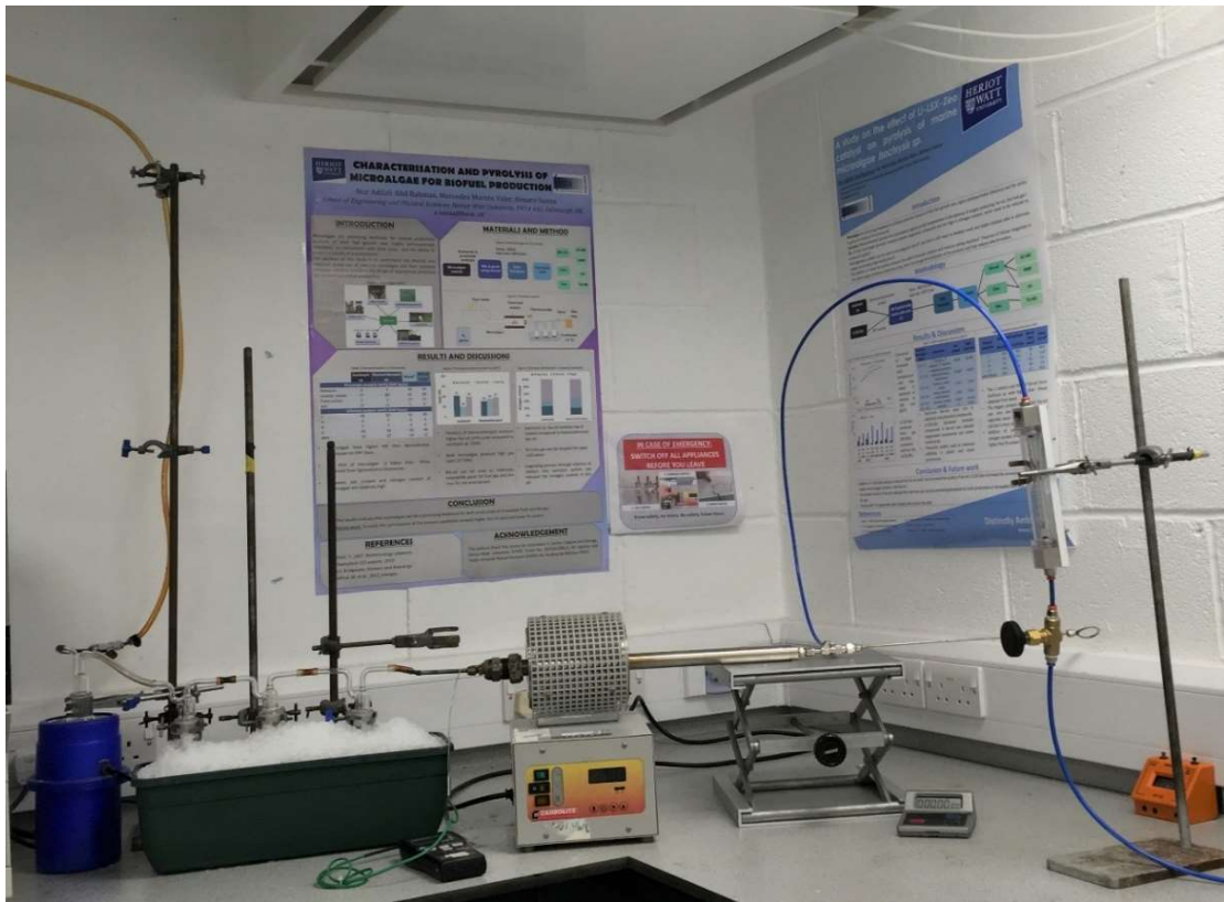
Figure 3-12 (a) Schematic diagram. (b) Real set-up of the horizontal pyrolysis
