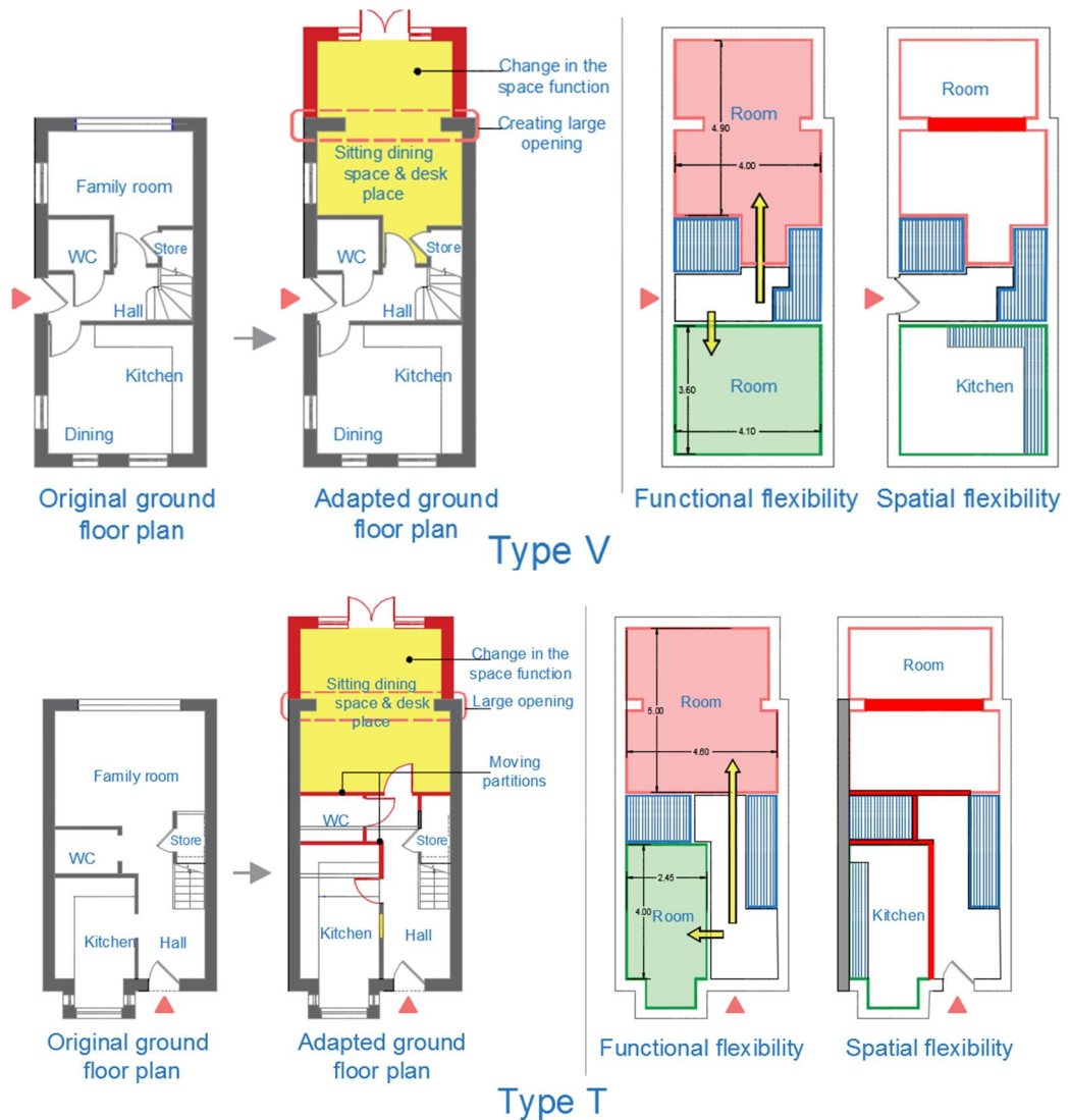
Figure 6.21: The layout arrangement of types T and V before and after extension. Source: the architects (id: Partnership Midlands), re-drawn and adapted by the researcher.
