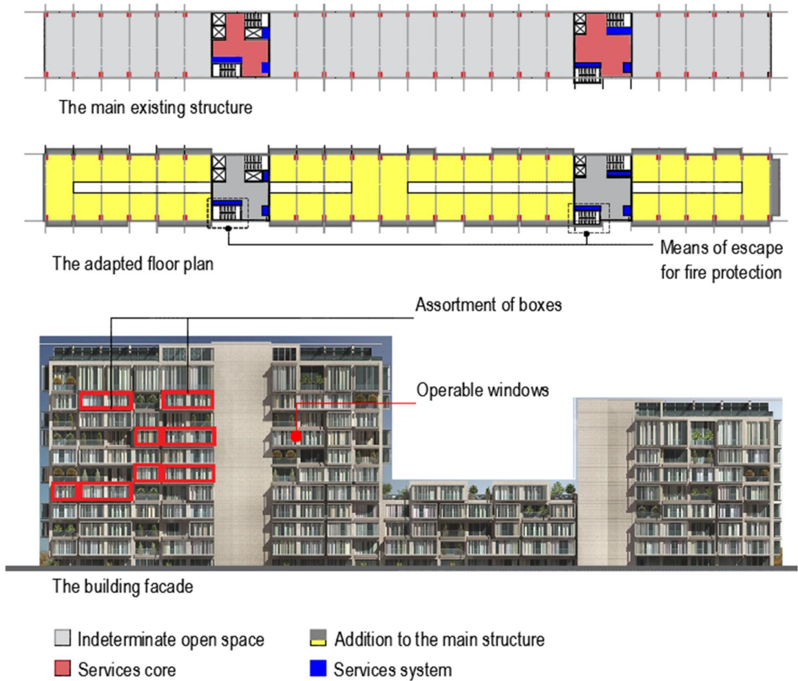
Figure 7.6: Flexibility in building use of the Levent loft 1 project. Source: the researcher.
