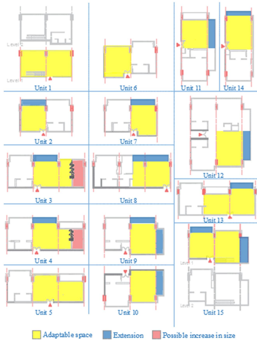
Figure 7.10: Different types of adaptable rooms in the Levent loft 1 project. Source: the researcher.
