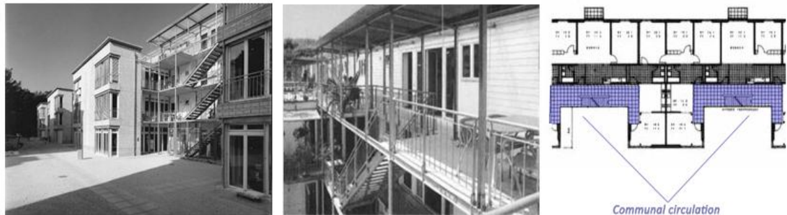
Figure 3.5: Hellmutstrasse. ADP-Architekten, Zurich, Switzerland, 1991, flexibility in communal circulation. Source: Leupen et al. (2005).
