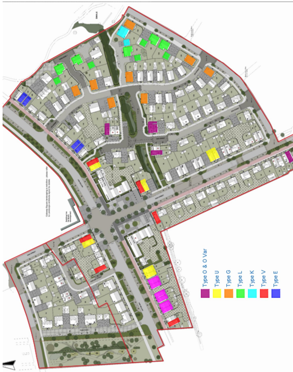
Figure 6.16: FEH types of Tattenhoe Park site 1 development. Source: the architects (id: Partnership Midlands) edited by researcher.
