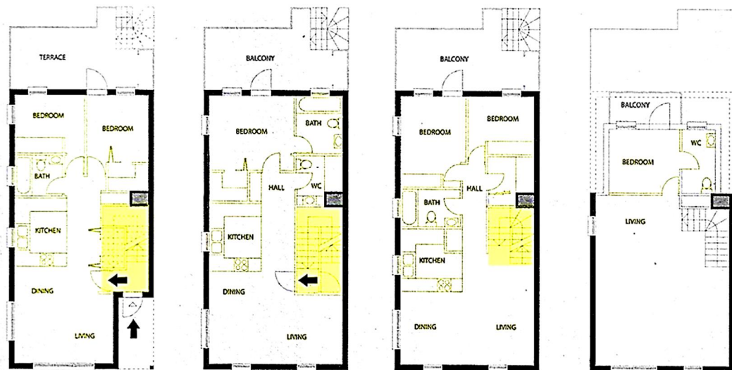
Figure 3.15: Next Home, Avi Friedman, Canada, 1996 flexibility through dividing up. Source: Schneider and Till (2007, p. 112), edited by the researcher.
