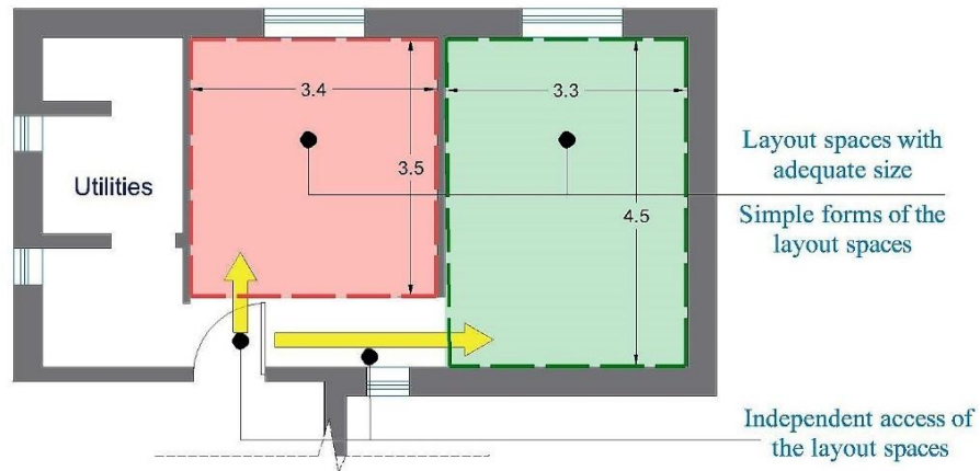
Figure 6.6 : Functional flexibility of the WLH. Source: the researcher.
