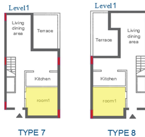
Figure 7.31: Flexibility in room function in the different units of the Eryaman Third Stage project. Source: the researcher.
