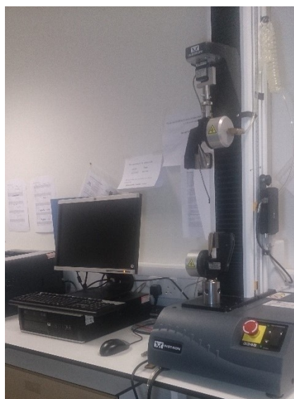
Figure 3-3 Instron Testing machine 3345K7484 based on dual-acting crosshead (up and down), Schematic diagram of Tensile Testing Machine.
