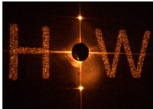
Figure 3-12 Experimental results of hologram and OAM superposition together when the wavelength of incident light is 600nm. a) LCP incidence b) RCP incidence.
