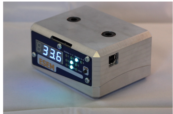
(b) Photograph of integration test-bed assembled within a translucent acrylic rapid-prototyped enclosure. The numerical display provides a live sensor reading, coupled with the LED matrix to the right which identifies the displayed sensor and measurement. A button enables cycling through the measurements.
