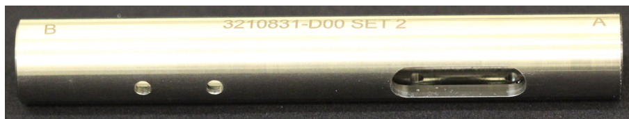
Figure 7.11: Photograph of manufactured bespoke multi-pass Herriott cell tube.
