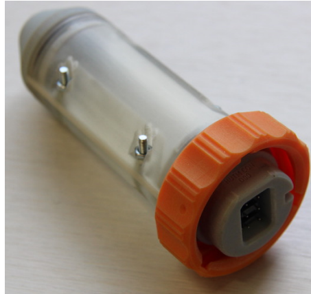
Figure 9.13: Photograph of cable-mounting umbilical connector assembled to verify mechanical operation.
