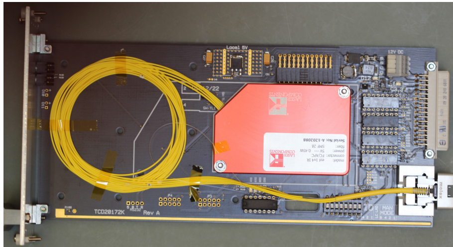
Figure 3.15: Photograph of assembled 1 \times 4 detector routing module. The module is dominated by the optical switch (red) and fibre routing (yellow).
