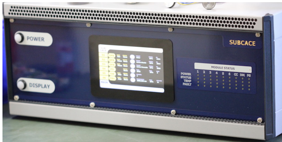
Figure 3.41: Photograph of medium-sized interrogation system that could support six diagnostic modules, one control card, and one PSU.
