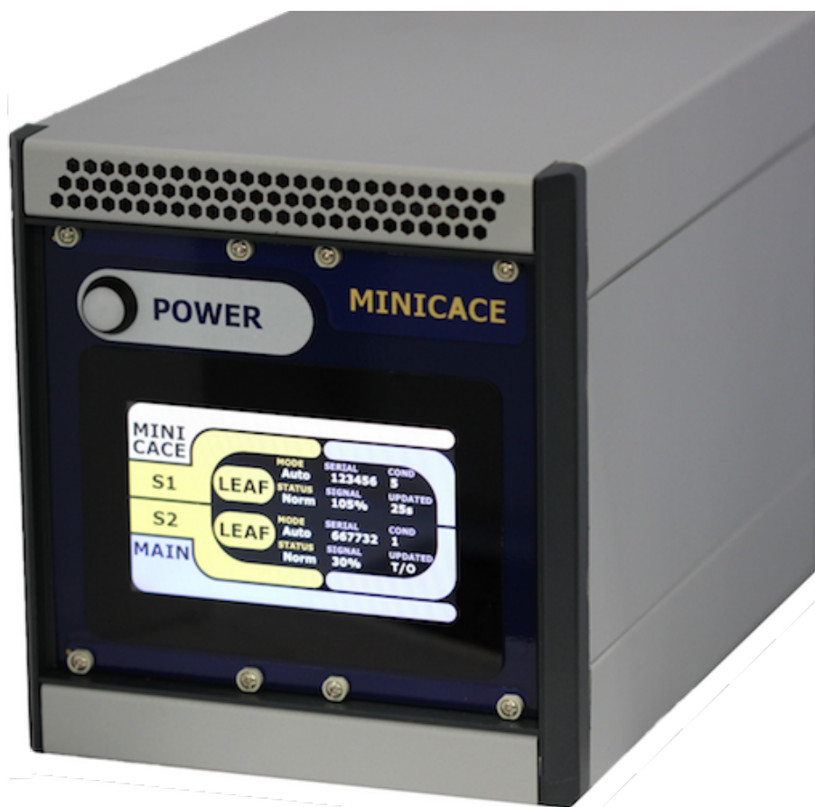
Figure 3.40: Photograph of smallest interrogation system design which could support two diagnostic modules and one control card.
