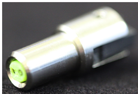
Figure 9.9: Photograph of assembled sensor package with the green sensor housing supporting two glass capillary tubes visible.
