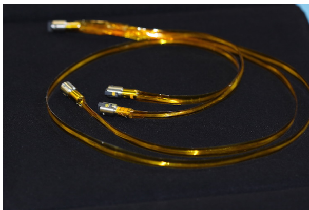
Figure 9.10: Photograph of encapsulated ribbonised optical fibre fitted with internal connectors and forming a 1 to 3 fibre fan-out.
