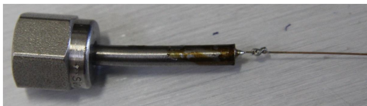
Figure 9.1: Photograph of solder seal optical fibre feed-through with Swagelok (USA) adaptor fitted for leak-testing.
