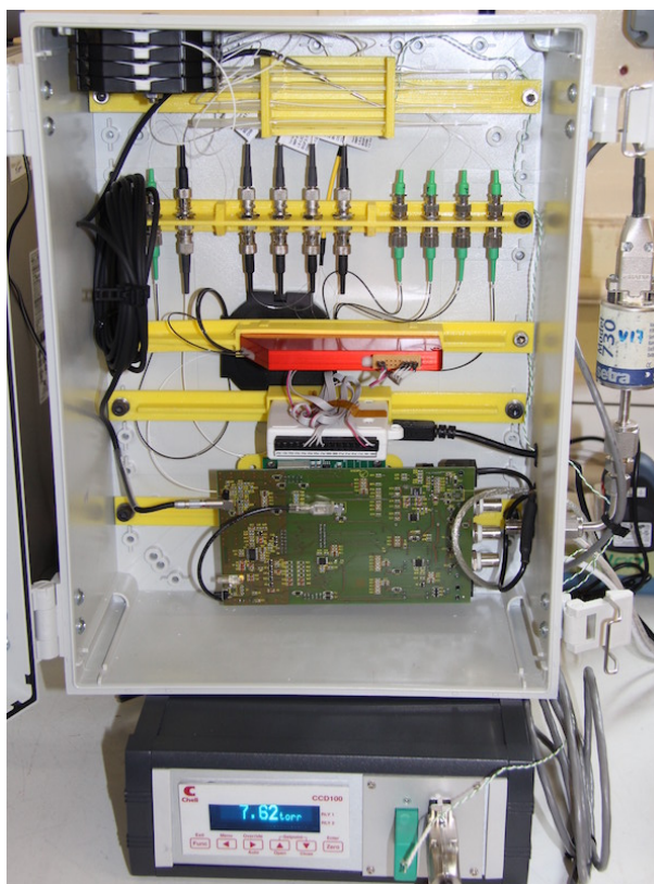
Figure 7.20: Photograph of the long-term oxygen sensor experimental configuration. The experiment was housed in a light-proof box.
