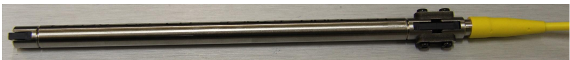
Figure 9.6: Photograph of fibre feed-through concept based around 8 mm Swagelok tubing and the bespoke internal connector design. Shown coupled onto a test breakout protected by a yellow plastic boot and furcation tubing.
