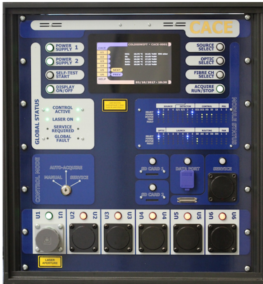
Figure 3.3: Front panel photograph of the interrogation system, featuring 8 primary dual-colour illuminated push-buttons, 10 secondary dual-colour illuminated push buttons, a full colour touch screen, four primary status dual-LED indicators, 128 module-status LED indicators, a three-position key-switch, two SD card slots, three electrical connectors, and optical fibre umbilical connectors.
