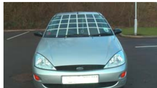
Fig. 3 Marking out 24 windscreen cells
