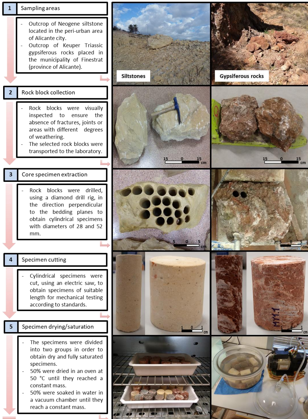
Figure 1. Rock block collection and specimen preparation.
