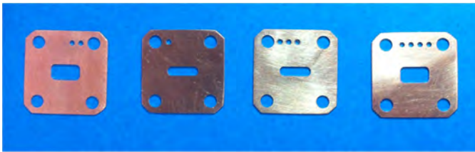
Fig. 21. View of the manufactured irises of the designed matching networks.
