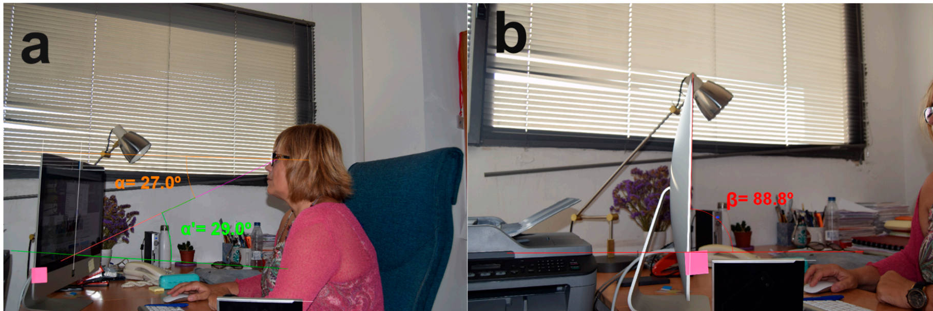
Figure 1. Drawing angles with QCad Trial 3.19.2 to calculate eye to screen angle \alpha , vision angle \alpha' (a) and screen tilt angle \beta (b).
