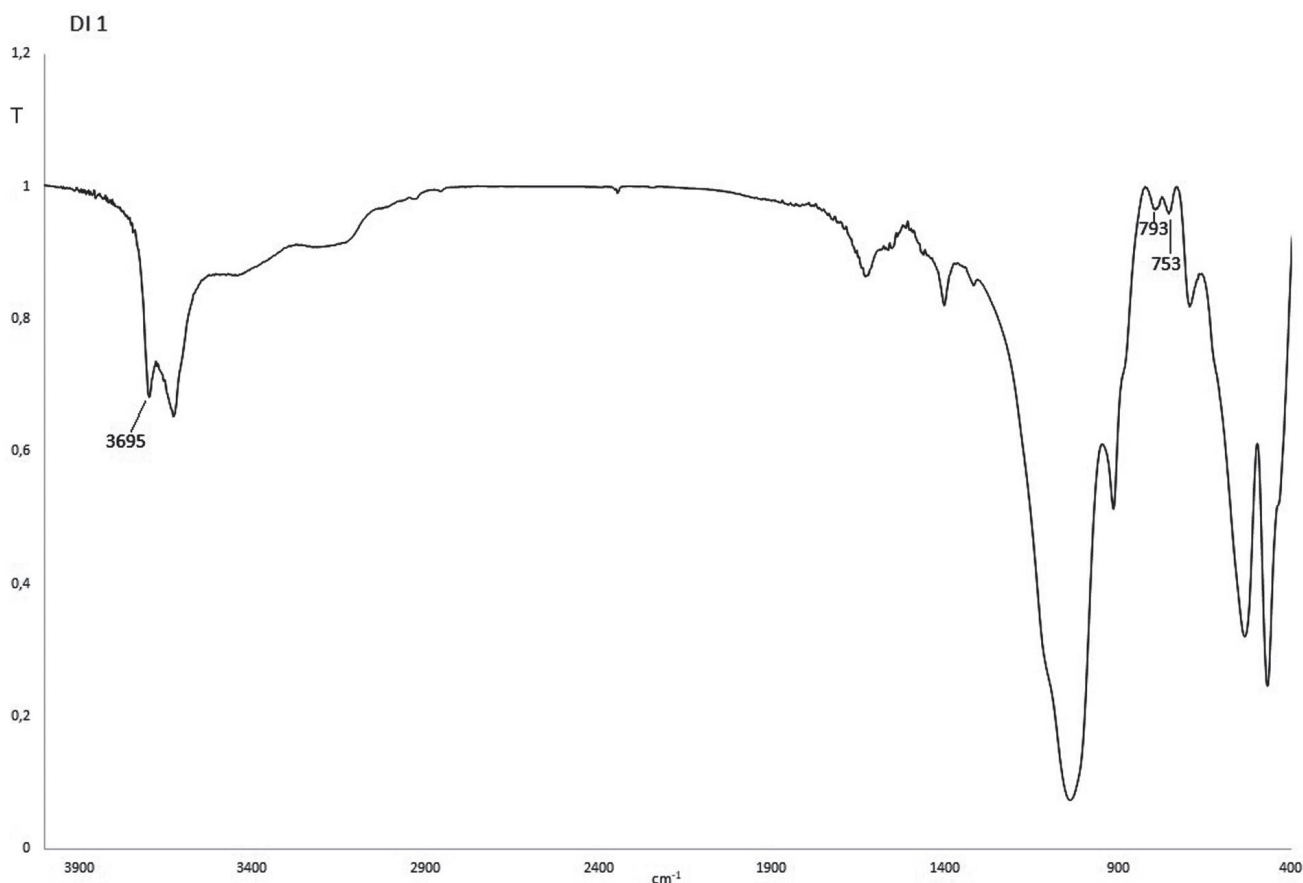
Figure 6. FTIR spectrum of DI1 (<2 μm) sample with wave numbers of bands showing presence of kaolinite.
