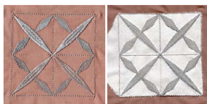
Fig.3 Front and back embroidery view with a two-coat torn interlining + one coat of sprayed interlining before cleaning
