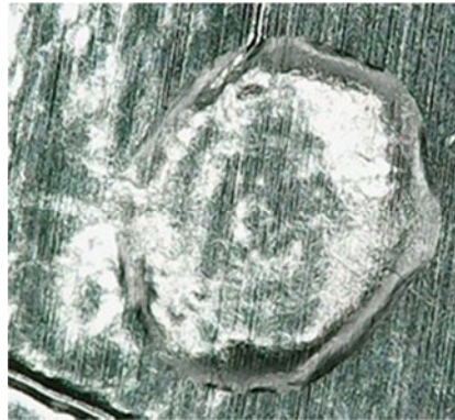
Fig. 9 Water traces on the aluminium surface that have remained after the cleaning process
