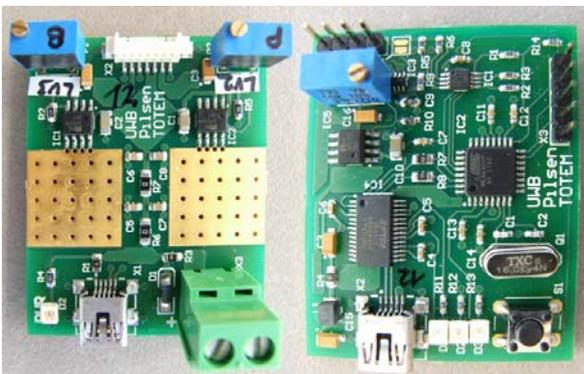
Figure 9. Accessory devices. The single board power supply (left) and TOTEM I2C interface (right).
