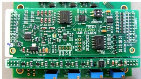
Figure 8. The remote access mezzanines. The U/I monitoring mezzanine (top) and the Remote Control mezzanine (bottom).
