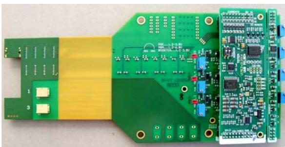
Figure 7. The Feedthrough board with mezzanines inserted in.
