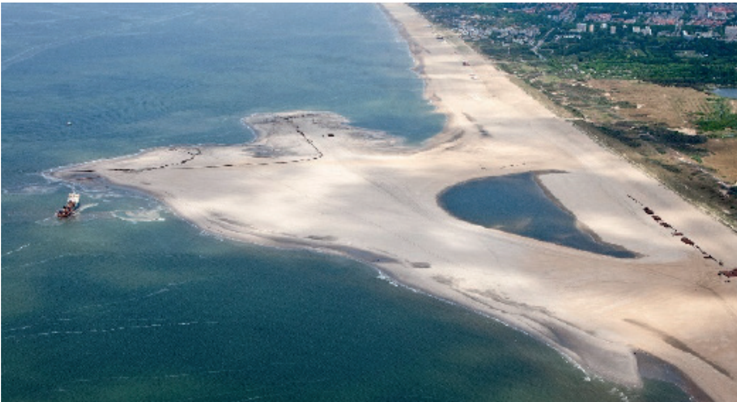
Figure 3.3. Sand engine on the Dutch coast ( https://oppla.eu/casestudy/17630 )
