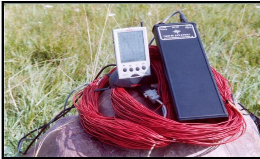
Figure 23. TDEM acquisition device, (adapted from [www.aerm.net](http://www.aerm.net)).
