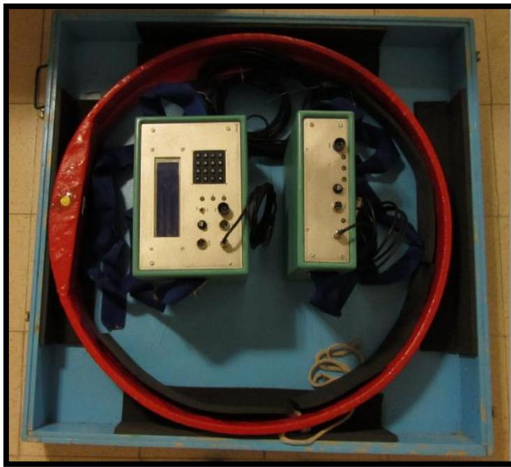
Figure 26. FDEM-8 (Des Barlow) – Coils (red), transmitter (right) and receiver (left).
