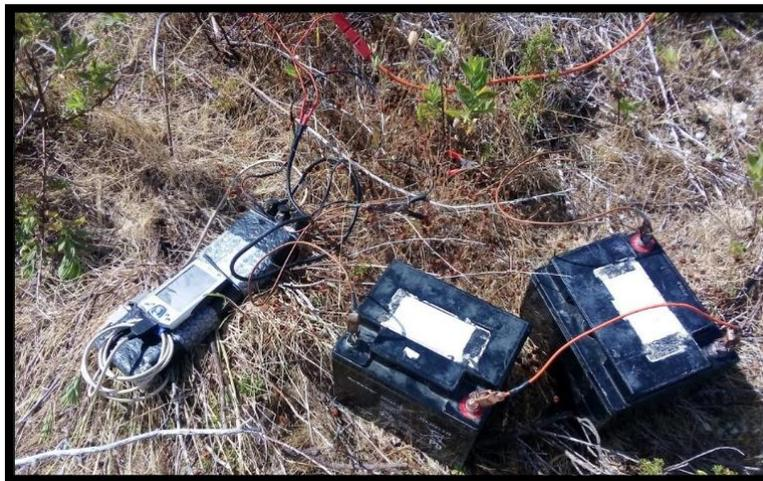
Figure 25. All components of the TEM-FAST connected to the main unit.
