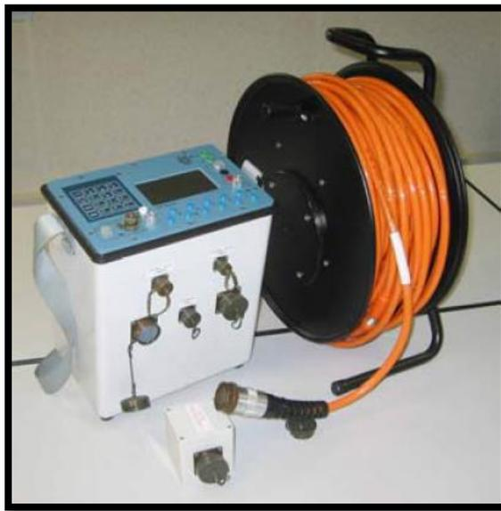
Figure 17. Syscal Pro Switch instrument (left) with a 90m coil (right) and a connection cube for coils.
