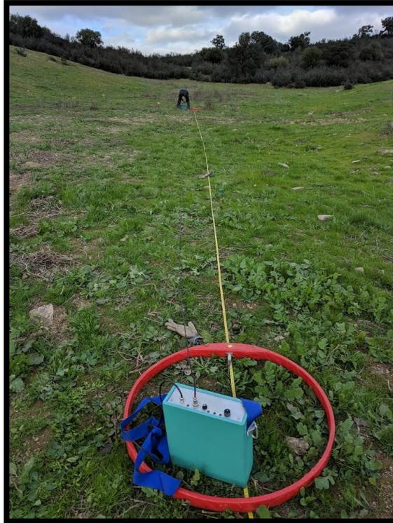
Figure 28. FDEM-8 sounding assembled.
