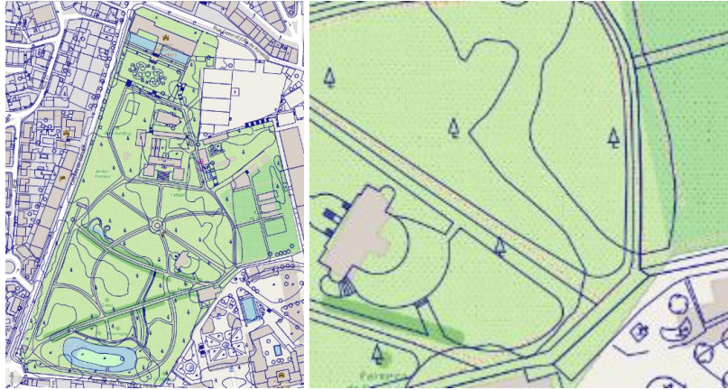
Figure 3.2. Overlay of geographical data onto OpenStreetMaps map. Overlaying of the map based on official geographical data from the botanical garden onto the map provided by open street maps. In the close up on the right we can better see that the paths provided by OpenStreetMaps (dotted orange), are slightly deviated from the correct paths (solid blue).
