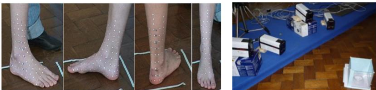
Figure 2.5 - Marker disposition on the foot-ankle complex (left) and capture system (right)[27].
