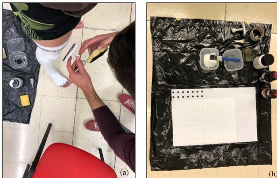
Figure 3.5 – Speckle pattern stamping (a) and painting/stamping equipment (b).
