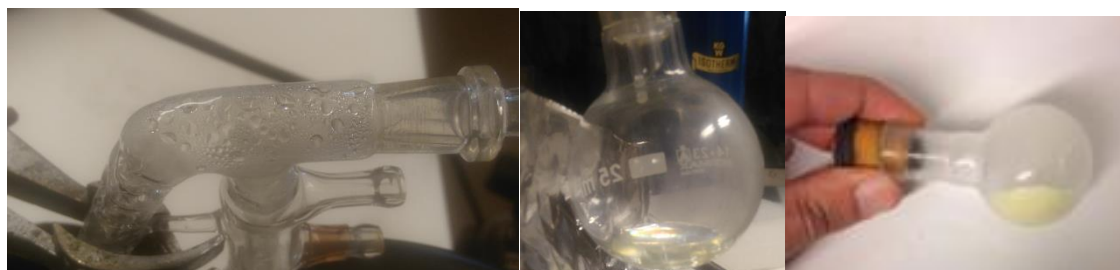
Figure 54 HMF vapour during the distillation in presence of \text{Na}_2\text{S}_2\text{O}_4 (left), freshly distilled 5-HMF (middle) and collected 5-HMF ( -12^\circ\text{C} ) (right)
