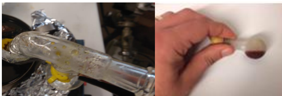
Figure 51 HMF vapour during the distillation without \text{Na}_2\text{S}_2\text{O}_4 (left) and collected 5-HMF ( -12^\circ\text{C} ) (right).
