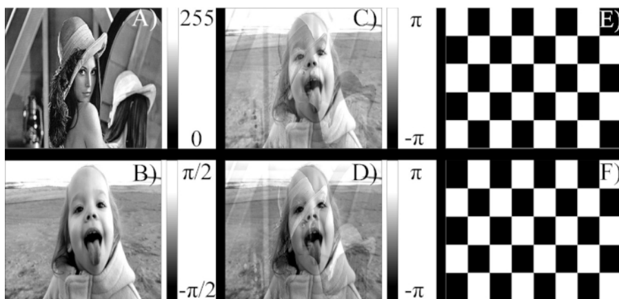
Figure 1: Computer generated patterns associated with the introduced encoding method. (A) User-defined amplitude pattern of the complex field. (B) User-defined phase pattern of the complex field. (C) Phase pattern corresponding to the first uniform wave in equation 1. (D) Phase pattern corresponding to the second uniform wave in equation 1. (E) First checkerboard pattern following the sampling process described with equation 4. (F) Second checkerboard pattern following the sampling process described with equation 4. Please click here to view a larger version of this figure.
