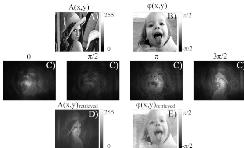
Figure 3: Representative experimental results under quasi-monochromatic illumination. (A) User-defined amplitude pattern of the complex field. (B) User-defined phase pattern of the complex field. (C) Interferograms associated with the polarization-based phase shifting technique developed in four steps and obtained after adding 0 , \pi/2 , \pi , and 3\pi/2 to the phase element \alpha(x,y) . (D) Retrieved experimental amplitude pattern. (E) Retrieved experimental phase pattern. Please click here to view a larger version of this figure.
