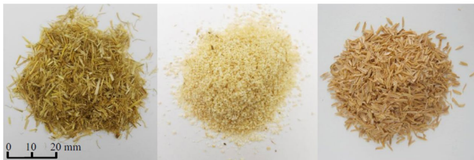
Fig. 1-6 Digital photos of natural fibers of barley straw, corn pith, and rice husk (from left to right) [34]
