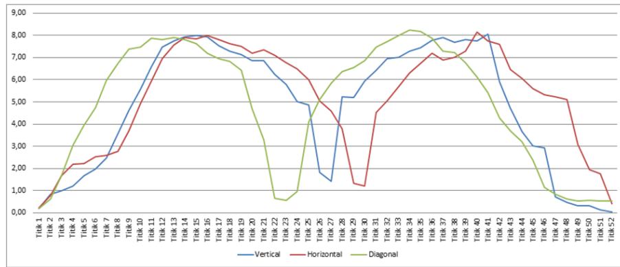
Figure 6 Wind velocity distribution curve before through flow straightener for measurement in vertical, horizontal, and diagonal position
