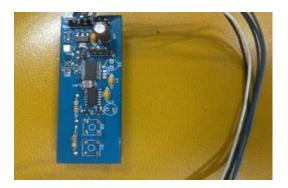
FIGURE 4.9bi Street Light Prototype for Streetlight Pole
