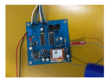
FIGURE 4.9a Street Light Prototype for the Main Board
