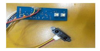
FIGURE 4.5 Diagram of the Infrared Sensor after soldering
