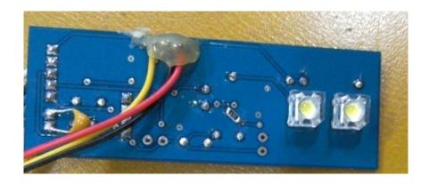
FIGURE 4.7 Diagram of the LED after soldering
