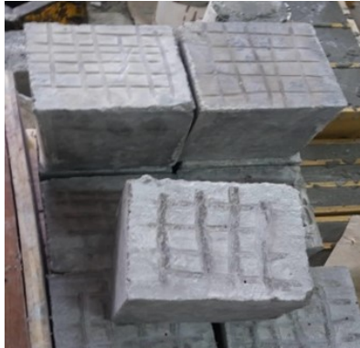
Figure 2 Roughness surface pattern of old PC specimens
