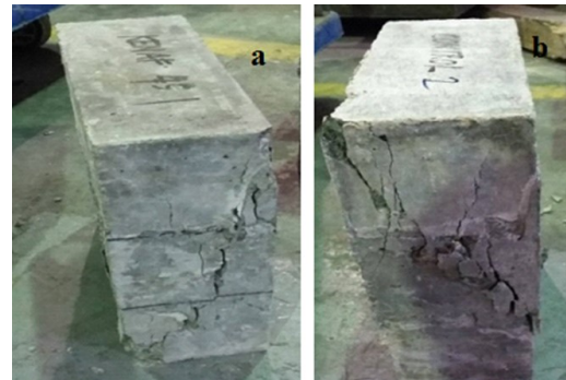
Figure 6 Interface failure mode of compression test sample (a) KFCC (b) PC
