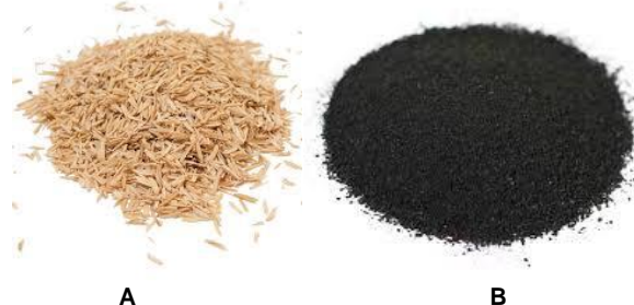
Figure 2 The physical illustration of rice husk (A) and rice husk ash (B).
