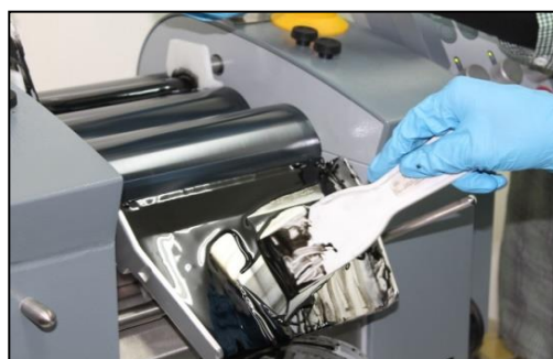
Figure 2 Dispersion process using three-roll mill machine
