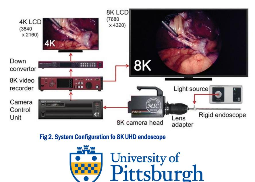
Achieve Realtime Abnormal Tissue Detection for Ultra High Definition (UHD) endoscopes with Machine Learning Algorithms and FPGA Computation Acceleration
