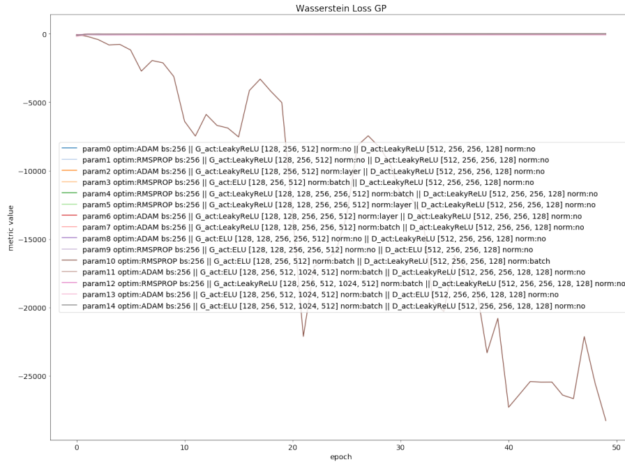
Figure 63: The Wasserstein GP loss is deteriorating for the run param10. The loss decreases up to -25000. Recall that the minmax WGAN optimization problem has the optimal value of zero. Batch normalization in the critic network seems to disturb the 1-Lipschitz continuity and hence should not be included in the critic network.
