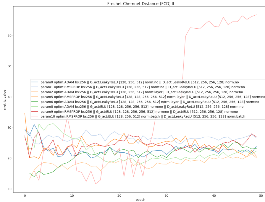
Figure 59: Including layer- or no normalization in the generator network leads to samples that do not minimize the FCD measure. param10 deteriorates over the training.
