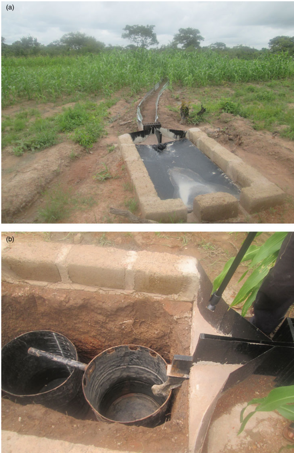
Fig. 3. (a) Structural layout of water runoff and erosion monitoring device and (b) water runoff collection chamber.
