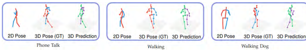
FIGURE 5.4: Visualization of 3D output of the estimation stage with some samples on the test set of Human3.6M (Ionescu et al., 2014). For each example, from left to right are 2D poses, 3D ground truths and our 3D predictions, respectively.
