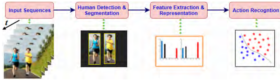
FIGURE 1.2: Overview of a typical video-based human action recognition system. The regions of interest (ROIs) corresponding to human motions are first identified. Their spatial-temporal features or descriptors, e.g. SIFT (Lowe, 2004), HOG/HOF (Dalal and Triggs, 2005; Laptev et al., 2008), HOG-3D (Klaser, Marszałek, and Schmid, 2008), are then computed and fed into a classifier for recognizing actions.
