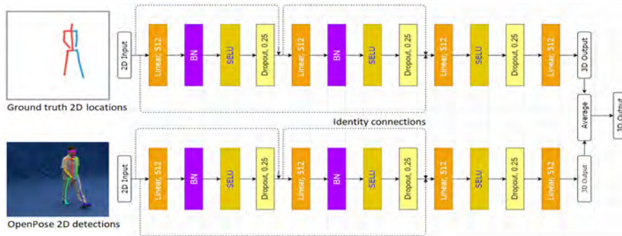
FIGURE 5.2: Diagram of the proposed two-stream network for training our 3D pose estimator.
