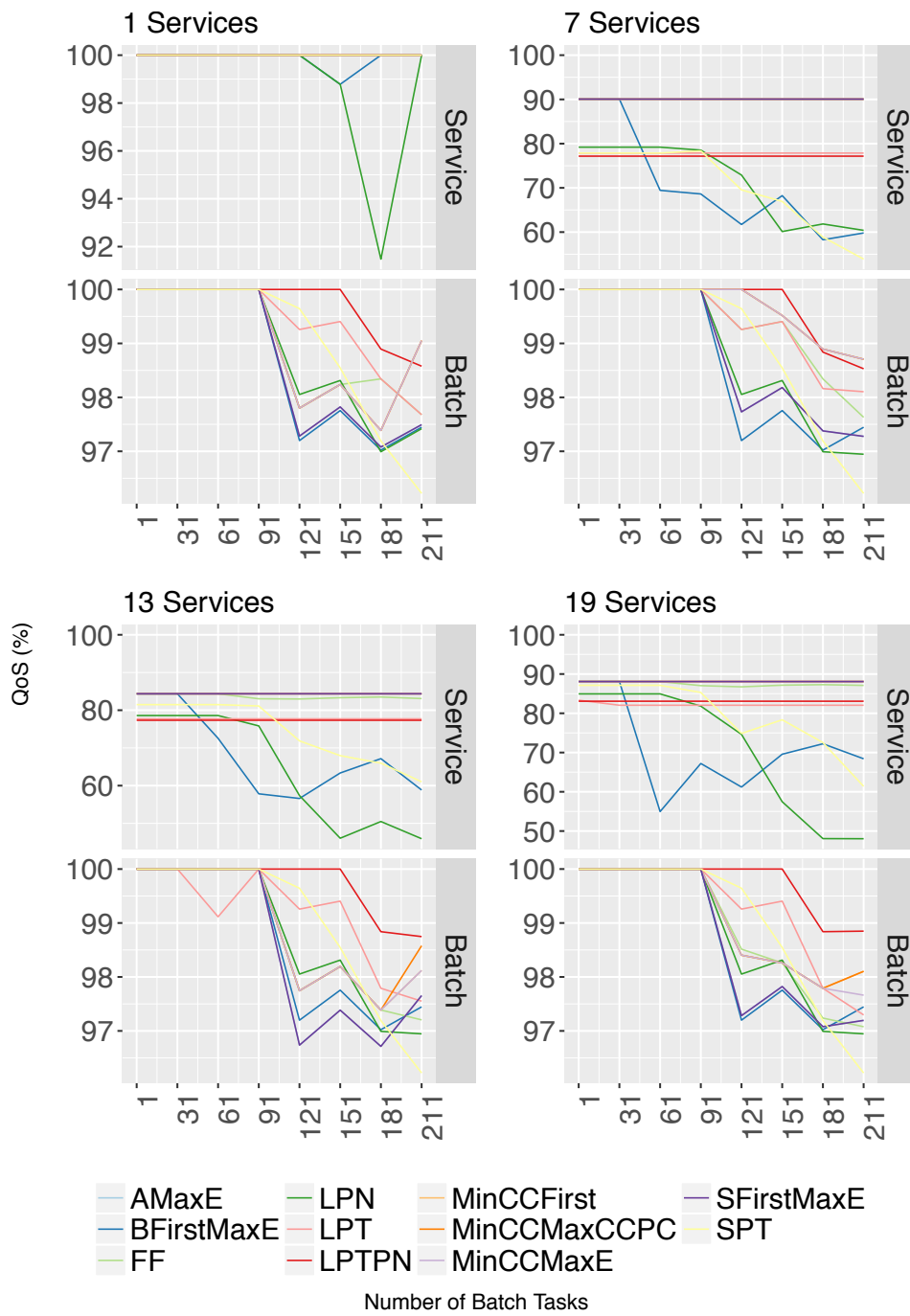
Figure 5.30: QoS distance of different algorithms for both batch and services over all workload variations with power profile 4.
