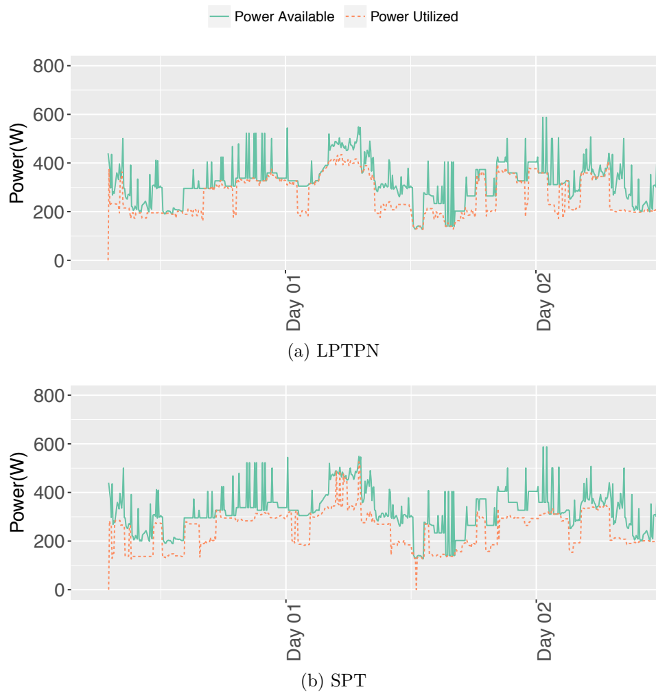
Figure 5.24: Power constraint and power consumption of workload with balanced profit for Batch and Service for LTPPN and SPT.
