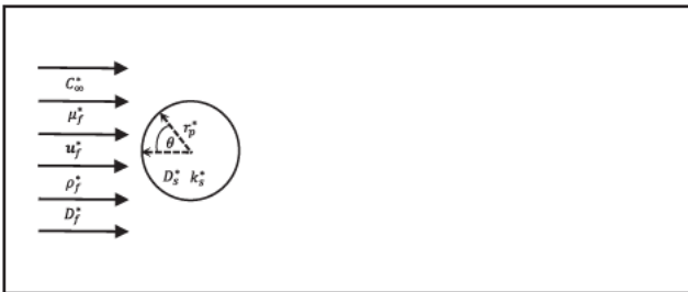
Fig. 7. Schematic diagram of the flow configuration and physical properties. The numerical domain size is L_x^* \times L_y^* = 100r_p^* \times 100r_p^* .
